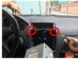
6. Remove the fixing screws of the original monitor, and take out the monitor
