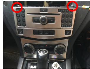
3. Remove the fixing screws of the original monitor
