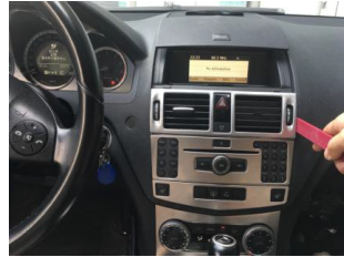
2. Pry the air conditioning vent panel
