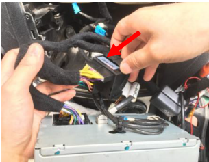
5. Unplug the original power harness from Host, and connect it to android harness.
