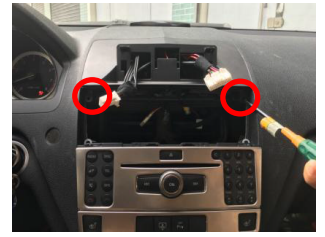
8. Assemble well the stand on original dashboard and put cables well
