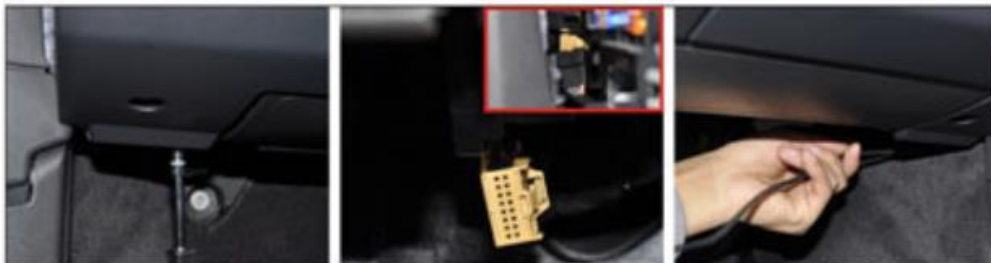
2. Remove the plate under steering wheel. Connect the CAN cable to the original PDC CAN cable. Go the cable to the glove box.
