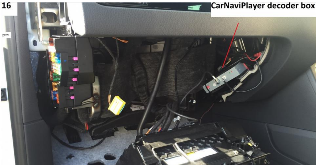
Box mounted behind centre console, secured with cable ties and sticky foam added to avoid any rattles
