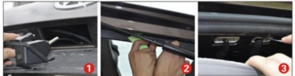
5. Install new tailgate handle camera and put the cable through your car.
