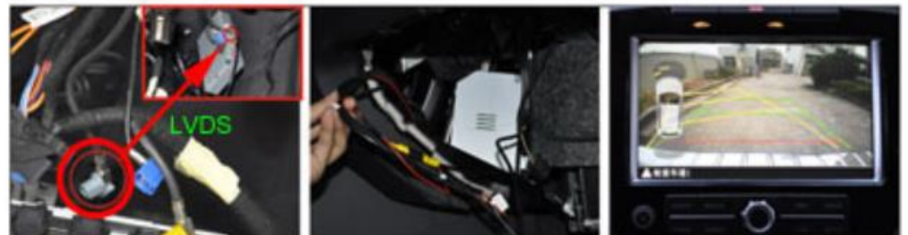
7. Connect the LVDS cable to interface box and connect the power cable as shown in the diagram wiring.
