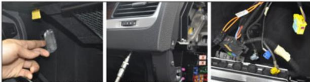
1. Remove the light in glove box, take the fuse box cover and take down glove box. (MUST NOT insert the key after unplug the yellow plug)
