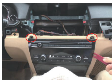
5.Remove the fixed screws, and take out the panel.
