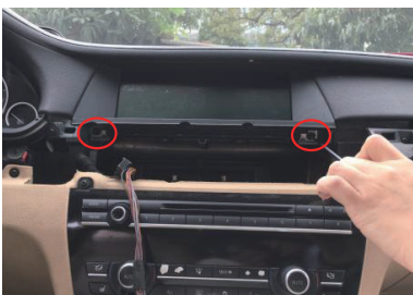
4.Remove the fixed screws from original monitor.
