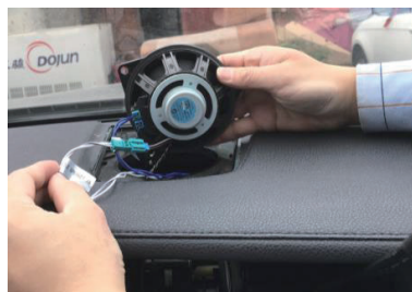
8.Connect well the center speaker cable with android cable.
