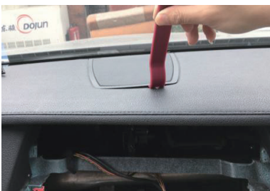
7.Pry loose the net and take out the center speaker.
