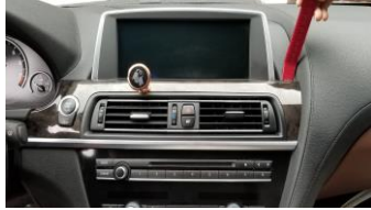
2. Loosen the right AC outlet.
