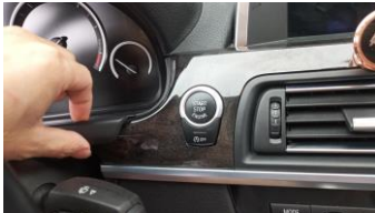
4. Remove the A/C outlet.
