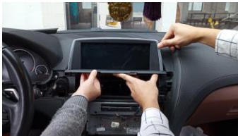
10. Remove the original screen.
