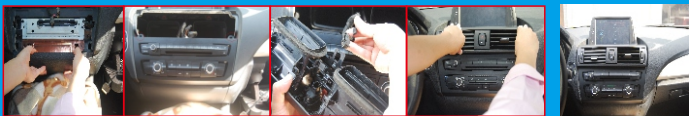
15 Put the air conditioning panel, panel, air conditioning vent back and plug all connectors, tighten the screws
