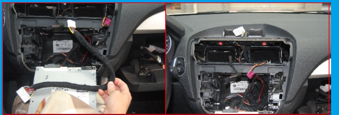
10 Plug the Head Unit and display screen connecting cable and GPS antenna
