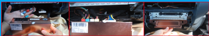
13 Plug all connectors and tighten the screws to fix the CD and head unit
