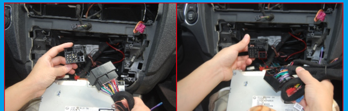
9 Unplug the original CD's connector, connect to our power cable, if there are fiber optic wires, please move to relevant PIN of our connector
