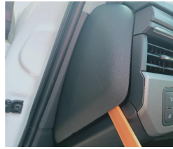
2. Pry open the main driver's side baffle
