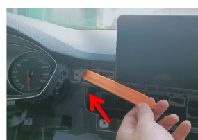
22. Use a pry knife to slightly loosen the original instrument and remove the original screen
