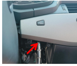
6. Remove the central control silver panel fixing screws
