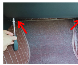
11. Remove screws on both sides of the bottom of the glove box and remove the glove box
