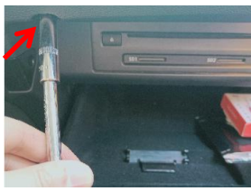
9. Open the glove box and remove the six holding screws
