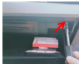
10. Remove the six holding screws
