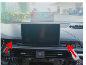
17. Remove the four fixing screws
